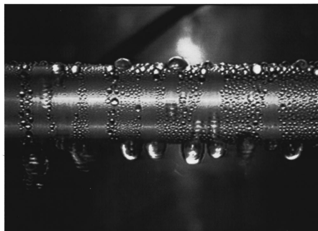
Fig. 6 Photograph of dropwise condensation on self-assembled monolayer (SAM) coated copper tube under atmospheric condition. Captured from condensation video.
